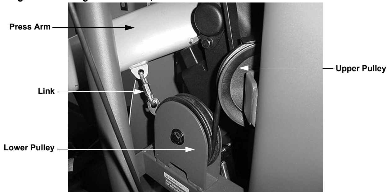
Diagram 4.79 - Right Press Arm, Rear View
