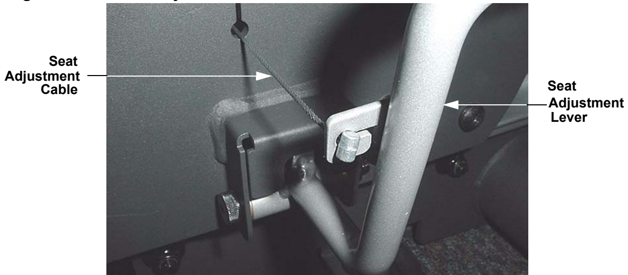
Diagram 4.62 - Seat Adjustment Lever
